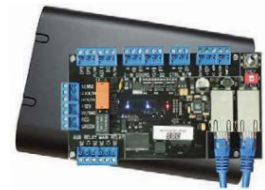
This PoE door controller can be installed and connected to a door access control system using ordinary Ethernet network cables, which facilitate power.
