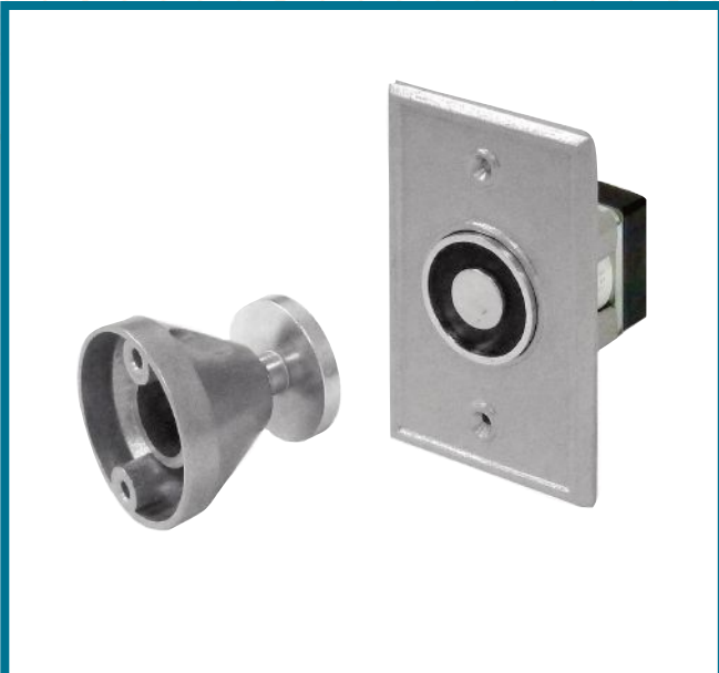
Electromagnetic door holders are designed to hold doors open and release the door by remote switch or fire life safety command center activation in a lockdown emergency. This simple combination should be used in conjunction with a mechanical door closer to ensure the door is fully closed when magnetically released.
