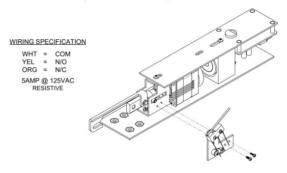
Route wires through the cable tie, along the side of the ELR and out.
